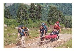
It is light weight and ergonomically designed with fully adjustable seating, footrests and armrests to assure comfort for both riders and "sherpas." A large-profile pneumatic tire rolls smoothly over all types of terrain. The TrailRider features a suspension system to ease the ride and a highly reliable disc brake system for increased safety. It has a cargo compartment for equipment and hiking gear. It is designed to fold down for ease of transportation and storage.
